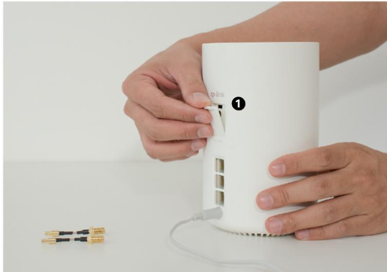
2. Insert the provided [SMB to SMA adapters](#) to the [External Antennas Ports](#), and then connect your LTE external antennas to the adapters.
